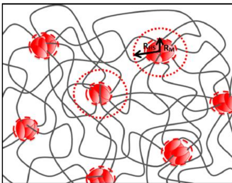
Fig. 1.4 Physically cross-linked network of PEG-DFA hydrogels; DFA hydrophobic aggregates (in red) and PEG chains (in black). R_{HS} is equivalent hard sphere radius according to Percus–Yevick model; R_M is mean micellar radius. [37]
