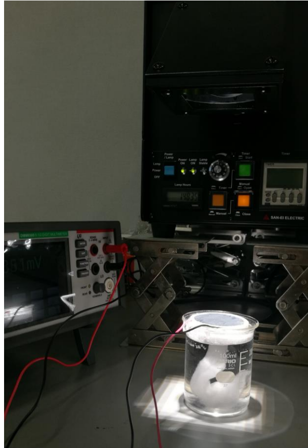
Fig. 5-19 Photograph of thermoelectricity generation setup and the electrical signal testing system.
