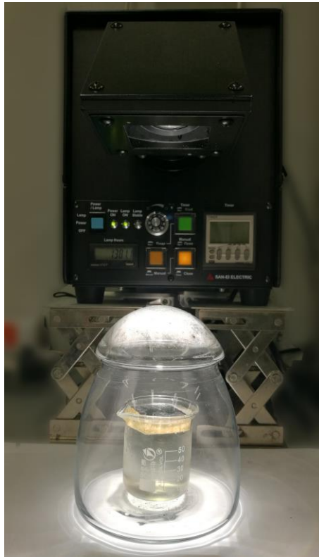
Fig. 4-9 Digital photograph of the PNPG wood solar evaporation system.
