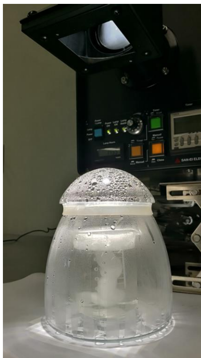
Fig. 5-16 Photograph of the homemade solar evaporation system under 1 sun for 3 h.
