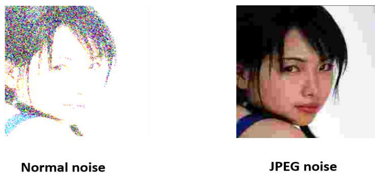
Figure 2.4: The results of Gaussian white noise N_G at different noise levels and JPEG compression noise N_{JPEG} .
