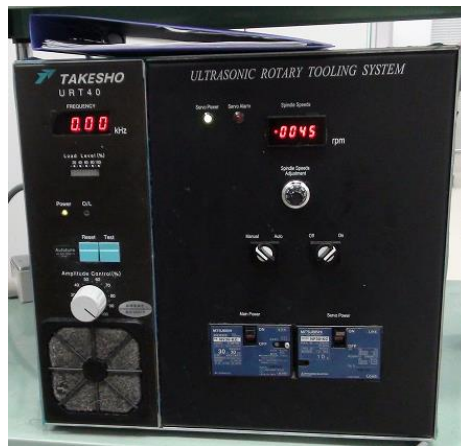
Fig. 2.4 Ultrasonic spindle controller
