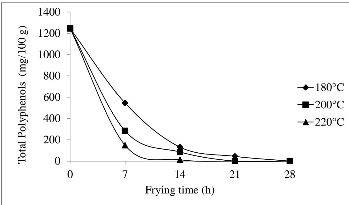
Figure 3-20 Changes in total polyphenols content of the EPKO during frying at different temperatures without oil replenishment.
