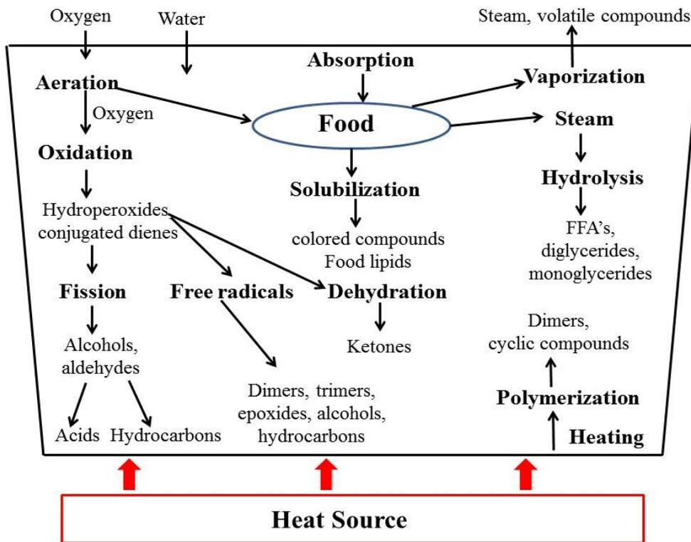
Figure 1-1 Physical and chemical reactions that occur during frying.
