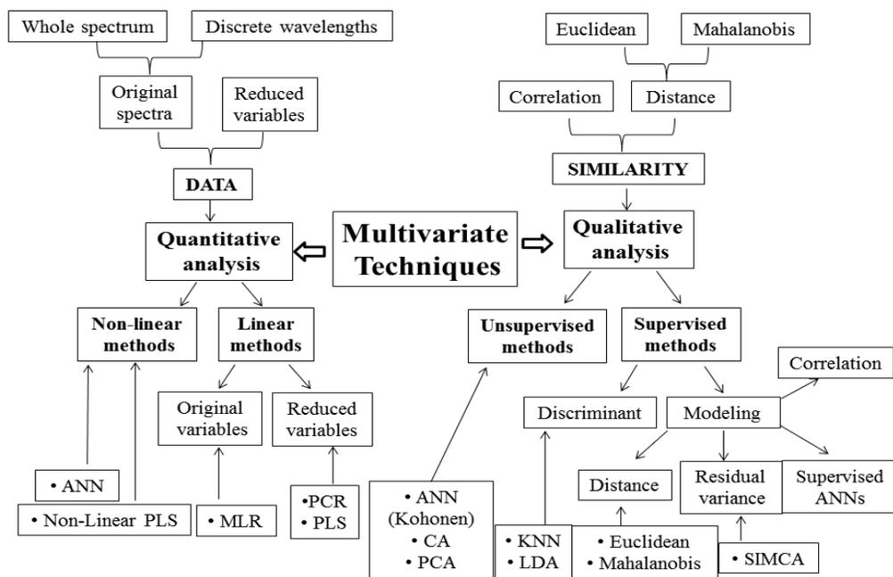
Figure 1-5 Classification of the major quantitative and qualitative multivariate analysis methods used in NIR spectroscopy.
