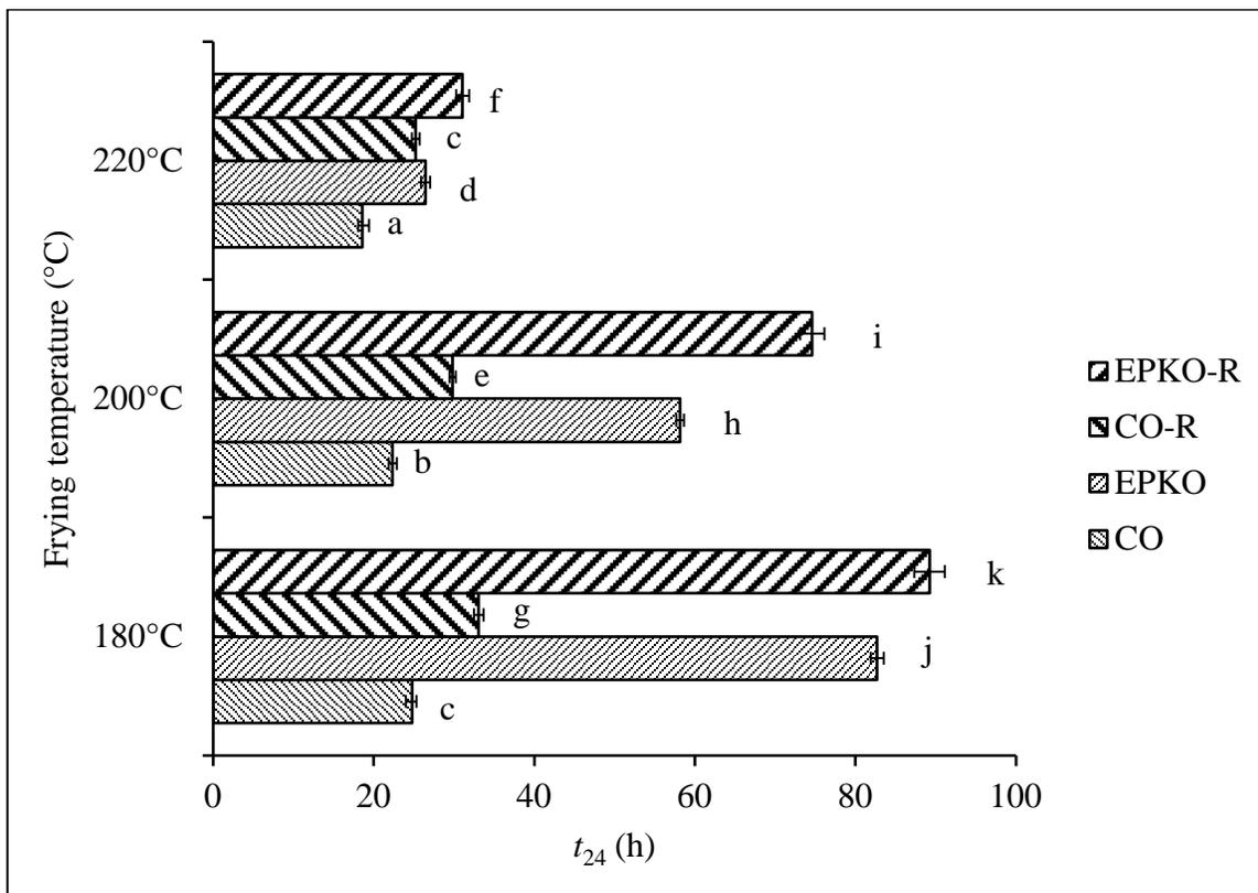
Figure 3-7 The time required to reach a TPC content of 24% ( $t_{24}$ ) for oil samples that were fried at different temperatures.
