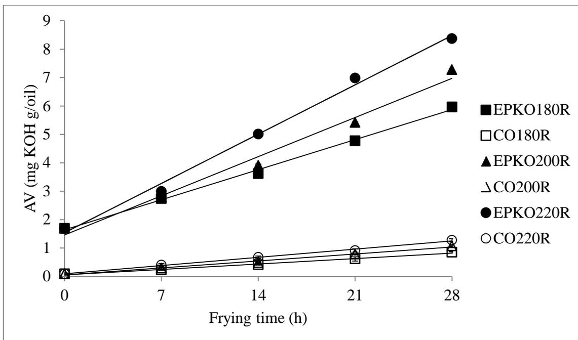
Figure 3-2 Changes in the AV during frying at different temperatures with oil replenishment.
