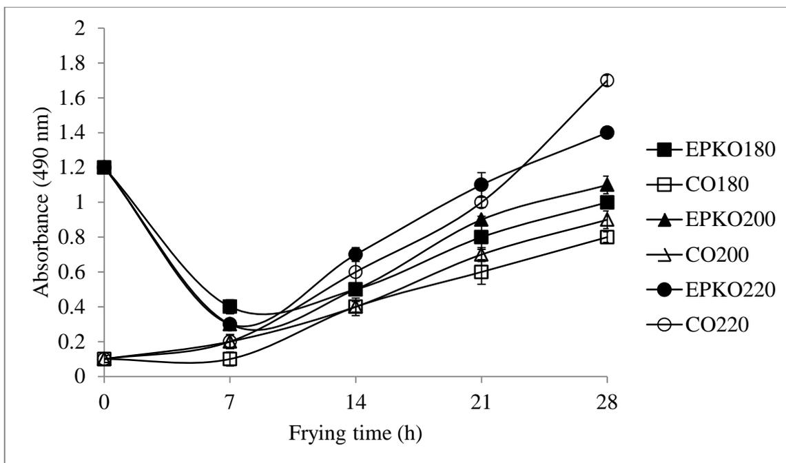
Figure 3-8 Changes in the color during frying at different temperatures without oil replenishment.
