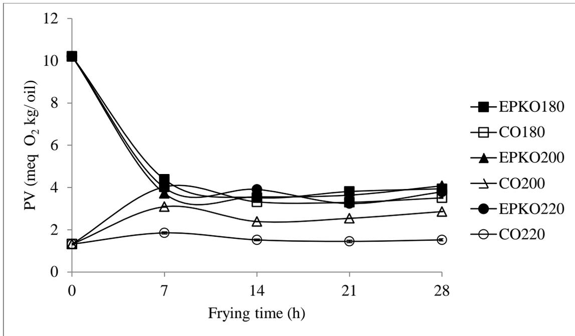
Figure 3-3 Changes in the PV during frying at different temperatures without oil replenishment.
