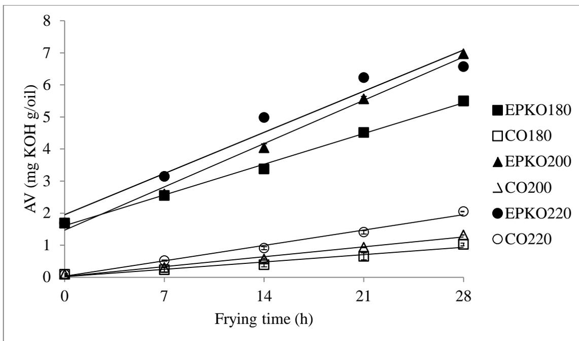
Figure 3-1 Changes in the AV during frying at different temperatures without oil replenishment.
