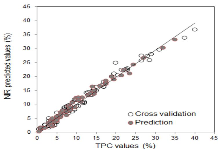
Figure 4-3 Scatter plot diagram comparing actual TPC values and NIR predicted values.
