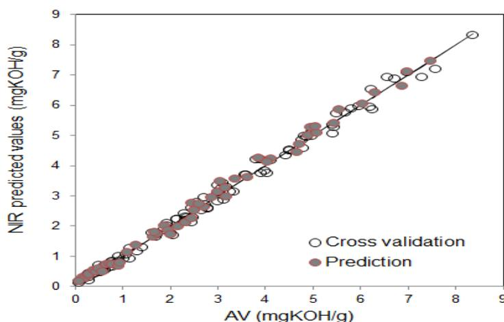
Figure 4-2 Scatter plot diagram comparing actual AV values and NIR predicted values.
