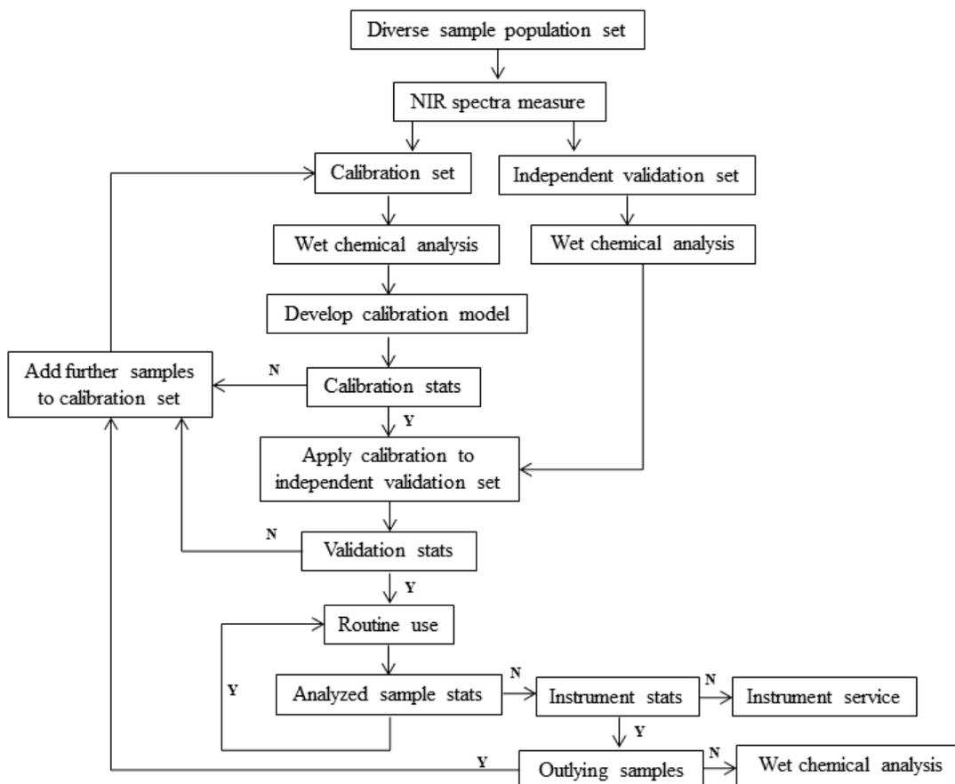
Figure 1-4 NIR spectroscopy calibration validation workflow.
