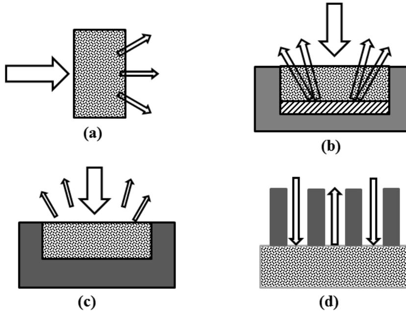
Figure 1-3 Modes of measurements employed in NIR spectroscopy.
