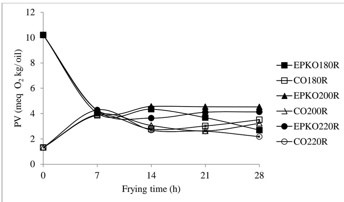
Figure 3-4 Changes in the PV during frying at different temperatures with oil replenishment.
