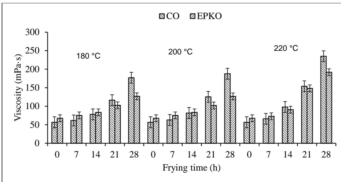
Figure 3-10 Changes in the viscosity during frying at different temperatures without oil replenishment.
