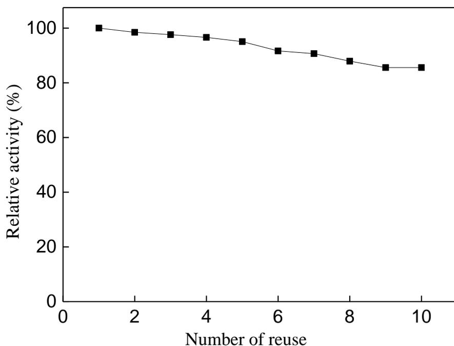
Fig. 3-9. Reusability of immobilized cellulase. CMC substrate was hydrolyzed by immobilized cellulase at 50 °C for 10 reaction cycles, each reaction time was 24 h
