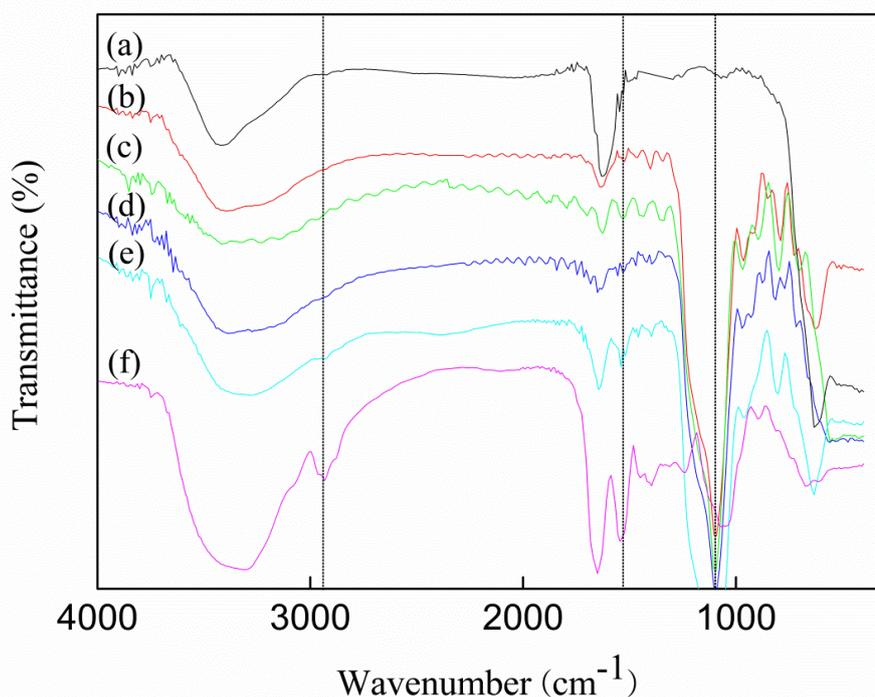
Fig. 3-5. FT-IR spectra of (a)  $\text{Fe}_3\text{O}_4$ , (b)  $\text{Fe}_3\text{O}_4/\text{SiO}_x$ , (c) FMS, (d) FMS-GA, (e) FMS-GA-EN and (f) EN. The FT-IR spectra of FMS nanospheres were investigated by the conventional KBr pellet method
