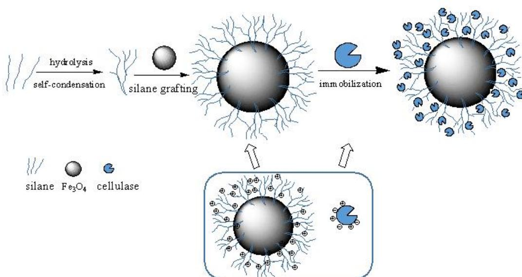
Scheme 4-1. Synthesis of functionalized magnetic silica nanospheres and immobilization of cellulase
