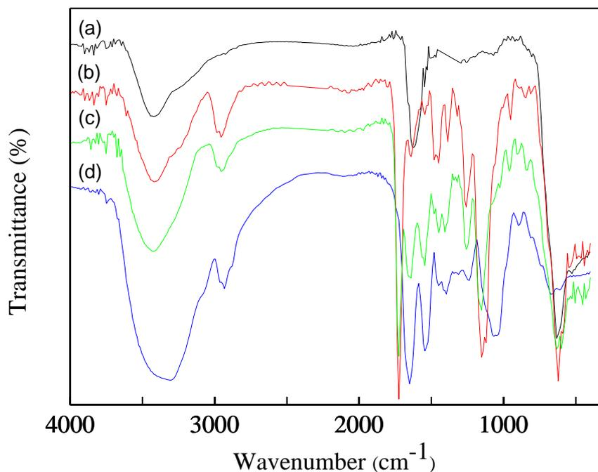
Fig. 5-2. FT-IR spectra of (a) Fe<sub>3</sub>O<sub>4</sub>, (b) Magnetic poly (GMA-MATAC), (c) Immobilized cellulase, (d) Cellulose
