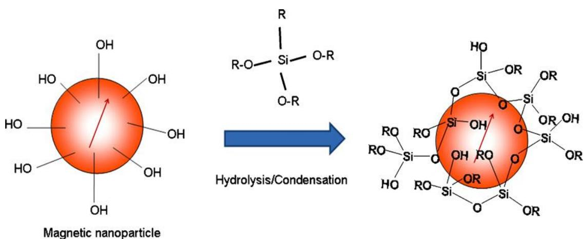
Fig. 1-7. Silane surface coating of a magnetic nanoparticle [62]
