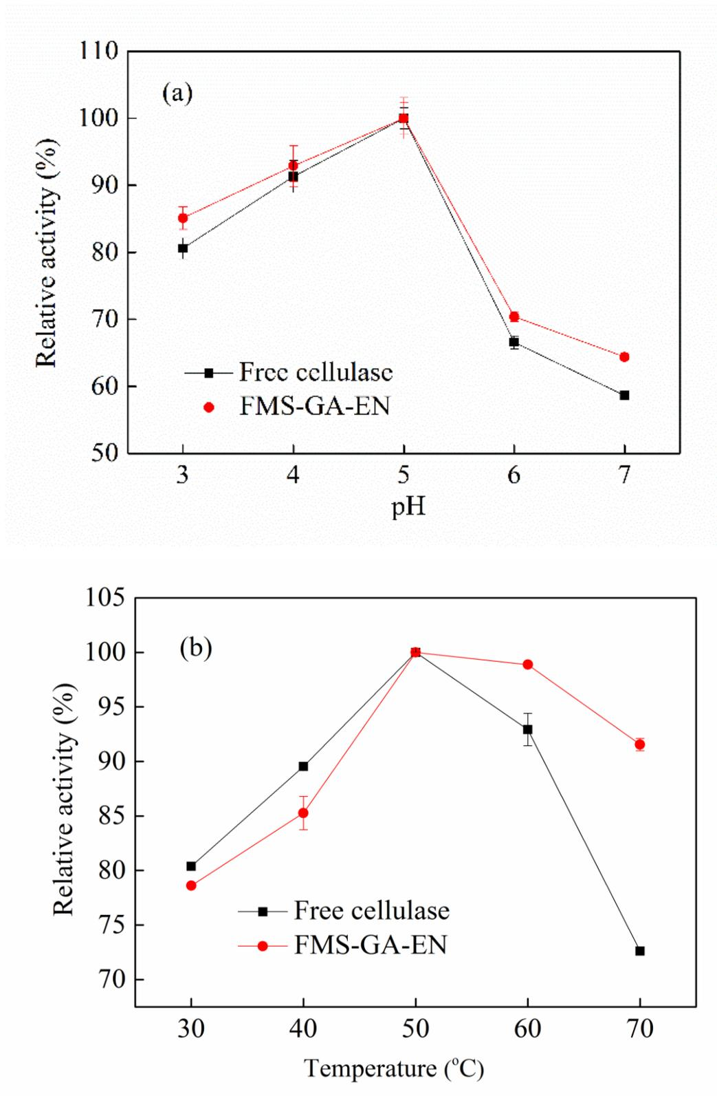
Fig. 3-7. Effects of pH and temperature on the activity of free cellulase and FMS-GA-EN: (a) pH and (b) temperature
