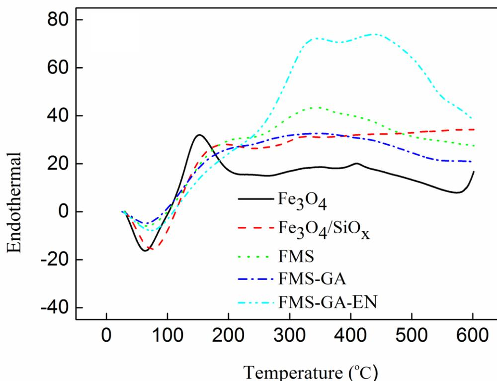
Fig. 3-6. DTA of  $\text{Fe}_3\text{O}_4$ ,  $\text{Fe}_3\text{O}_4/\text{SiO}_x$ , FMS, FMS-GA and FMS-GA-EN. Samples were heated from room temperature to 600 °C with a scanning rate of 10 °C/min in flowing nitrogen gas
