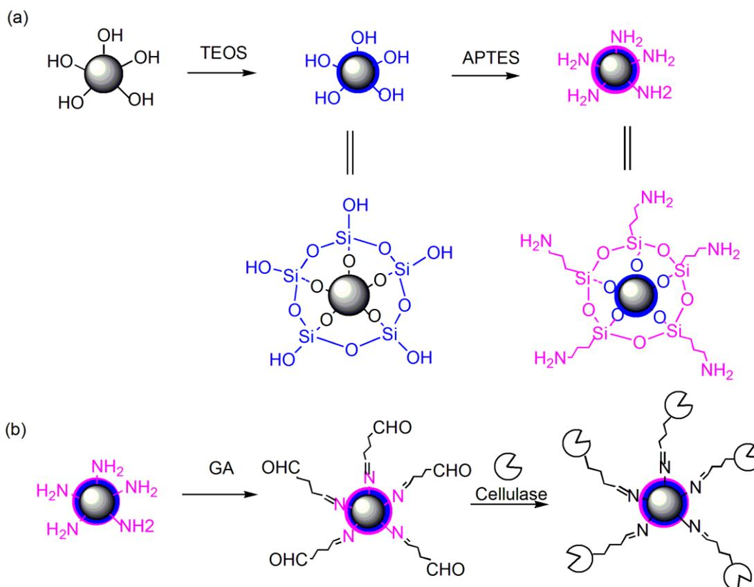
Scheme 3-1. (a) Synthesis of functionalized magnetic silica nanospheres and
