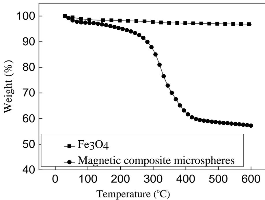
Fig. 5-3. TGA of Fe<sub>3</sub>O<sub>4</sub> and magnetic composite microspheres
