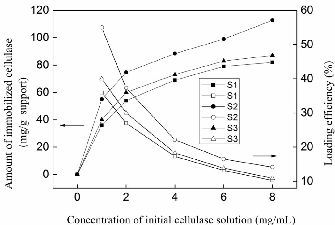
Fig. 4-6. Effect of concentration of initial cellulase on the amount of immobilized cellulase (solid) and loading efficiency (open)
