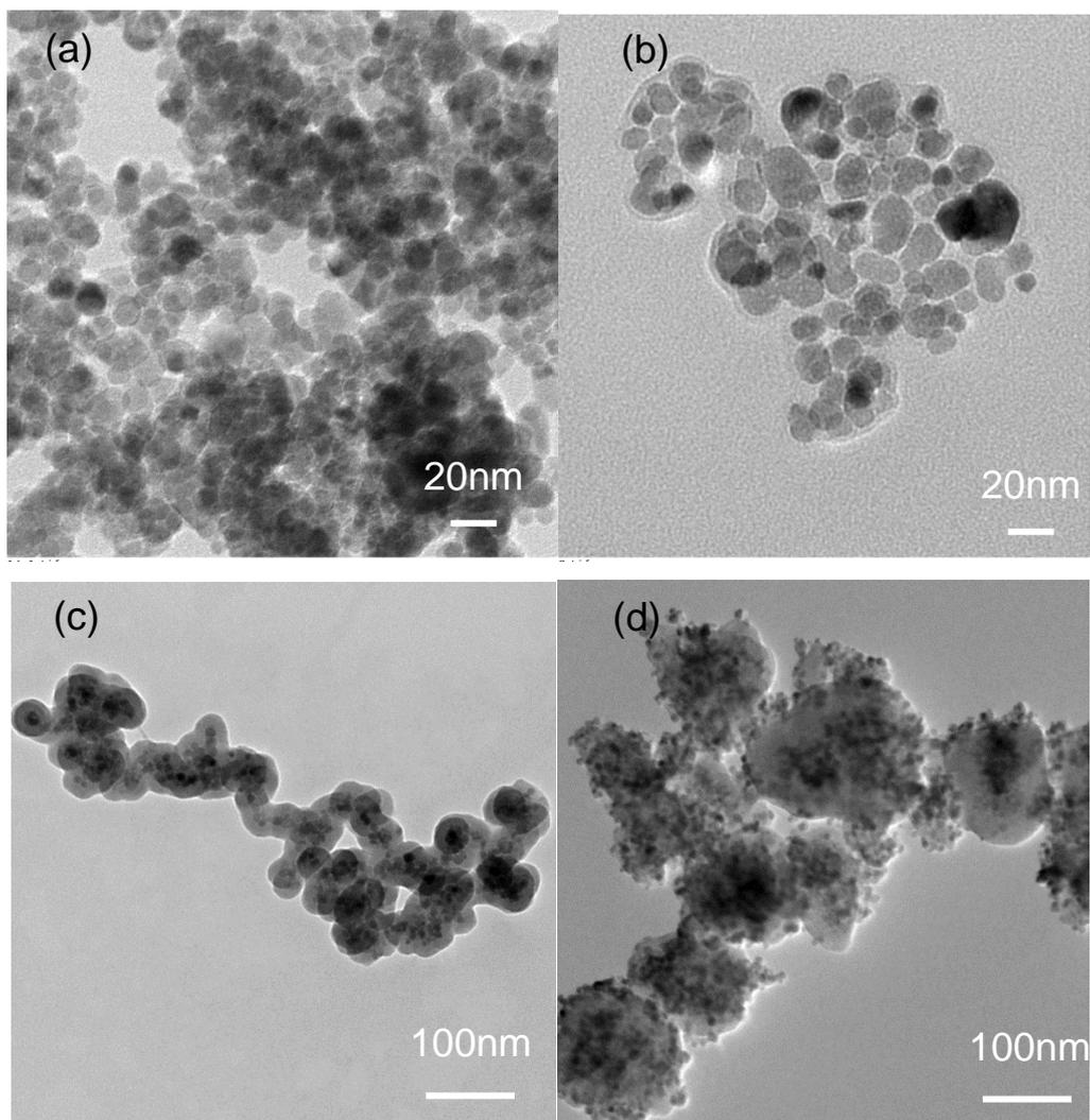
Fig. 3-1. TEM image of (a)  $\text{Fe}_3\text{O}_4$  and  $\text{Fe}_3\text{O}_4/\text{SiO}_x$  prepared with different amounts of TEOS: (b) MS<sub>3</sub>, (c) MS<sub>5</sub>, and (d) MS<sub>7</sub>.
