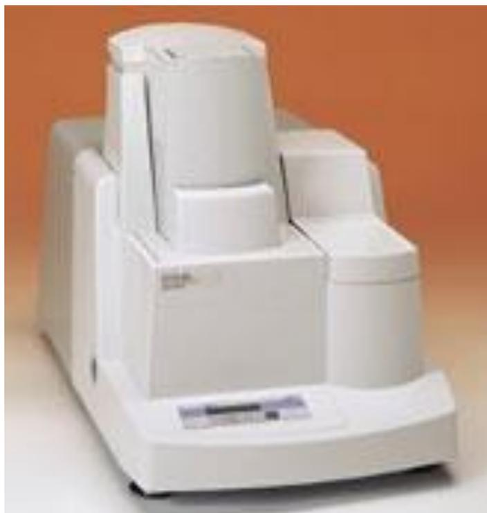
Fig. 2-4 TGA test machine
