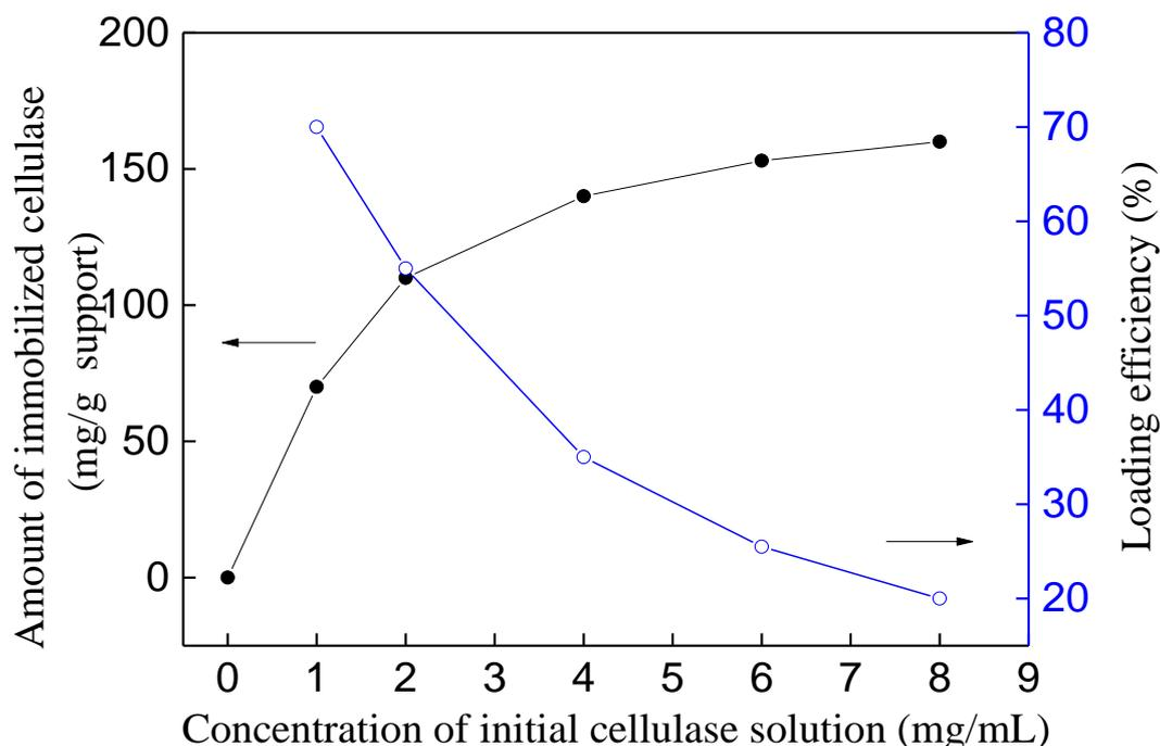
Fig. 5-6. Effects of concentration of initial cellulase solution on the amount of immobilized cellulase and the loading efficiency
