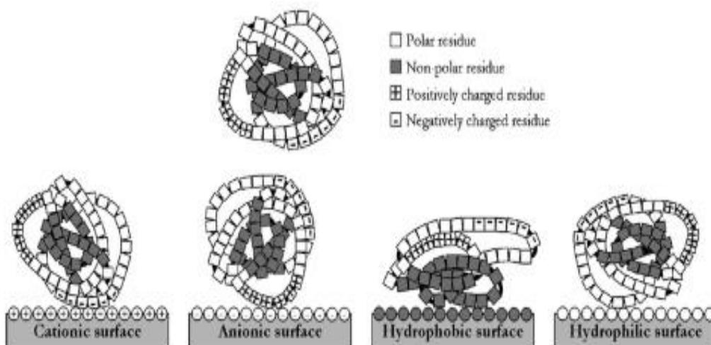
Fig. 1-3. Mechanisms of protein adhesion [30]
