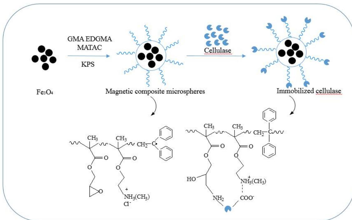
Scheme 5-1. Synthesis of the magnetic composite microspheres and immobilization of cellulase
