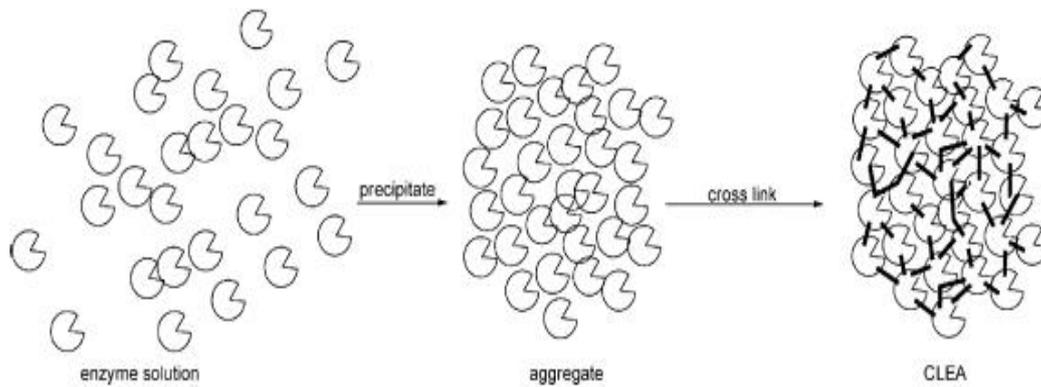
Fig. 1-4. Aggregation and crosslinking of an enzyme to prepare a CLEA [23]
