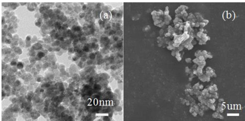
Fig. 5-1. (a) TEM image of  $\text{Fe}_3\text{O}_4$ , (b) SEM image of magnetic composite microspheres
