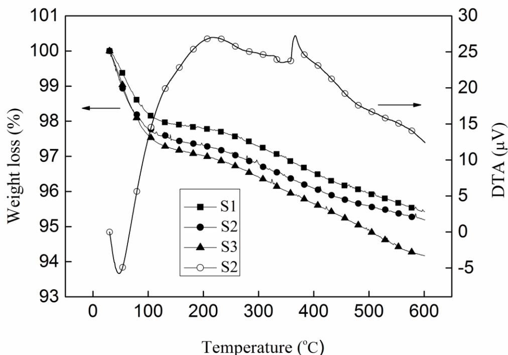
Fig. 4-3. Thermal analysis of three functionalized magnetic nanospheres: TGA of S1, S2 and S3 (solid); and DTA of S2 (open)
