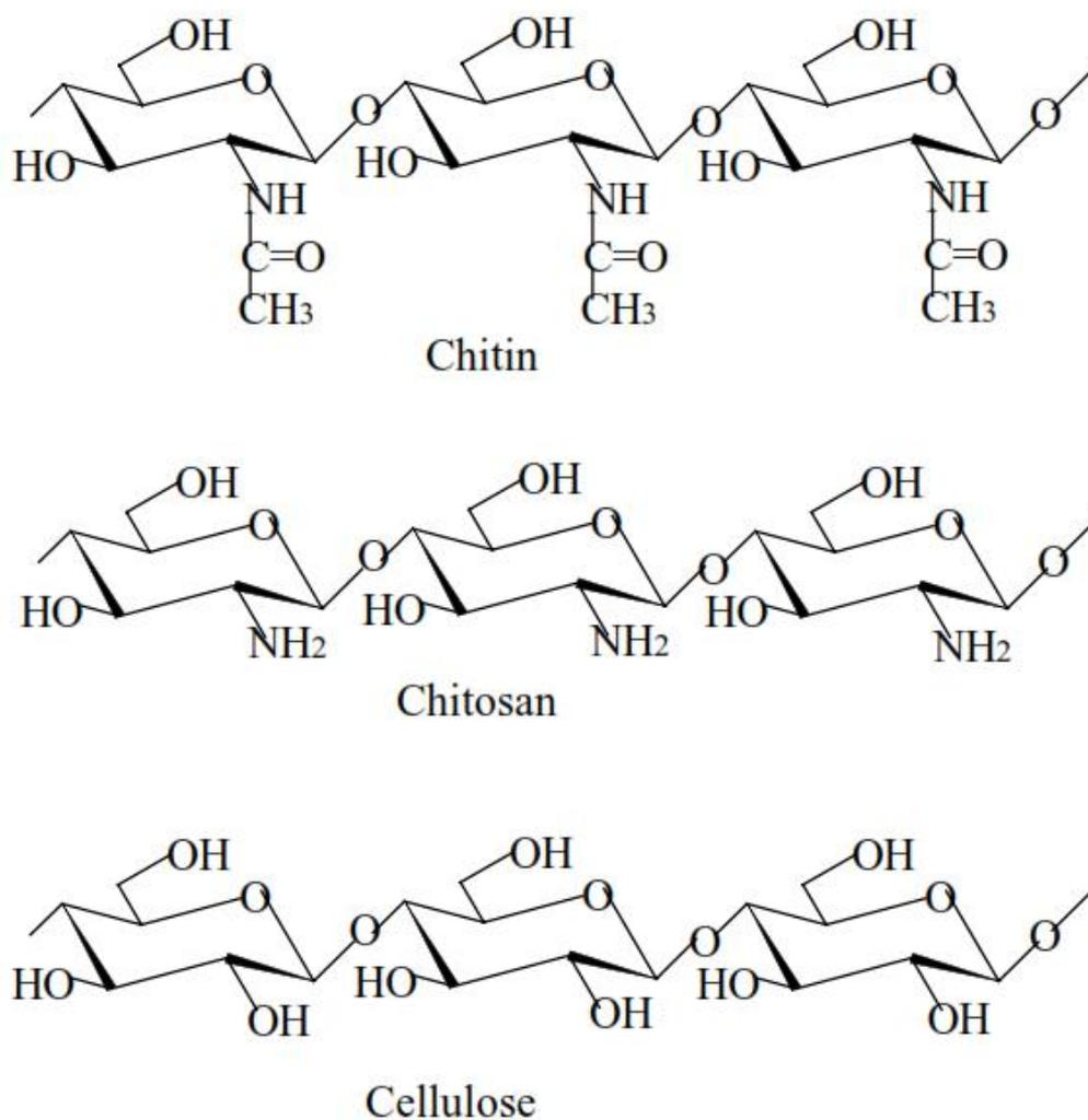
Fig. 1-8. Structure of chitin, chitosan and cellulose [70]
