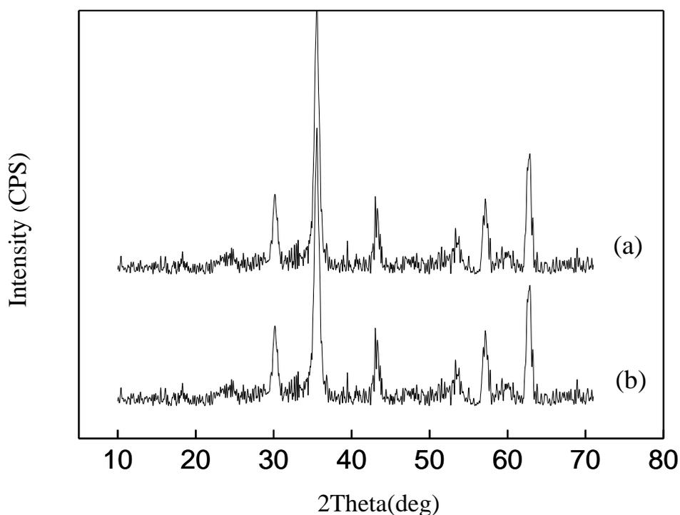
Fig. 5-5. Wide-angle X-ray diffraction patterns of (a)  $\text{Fe}_3\text{O}_4$ , (b) magnetic poly (GMA-MATAC)
