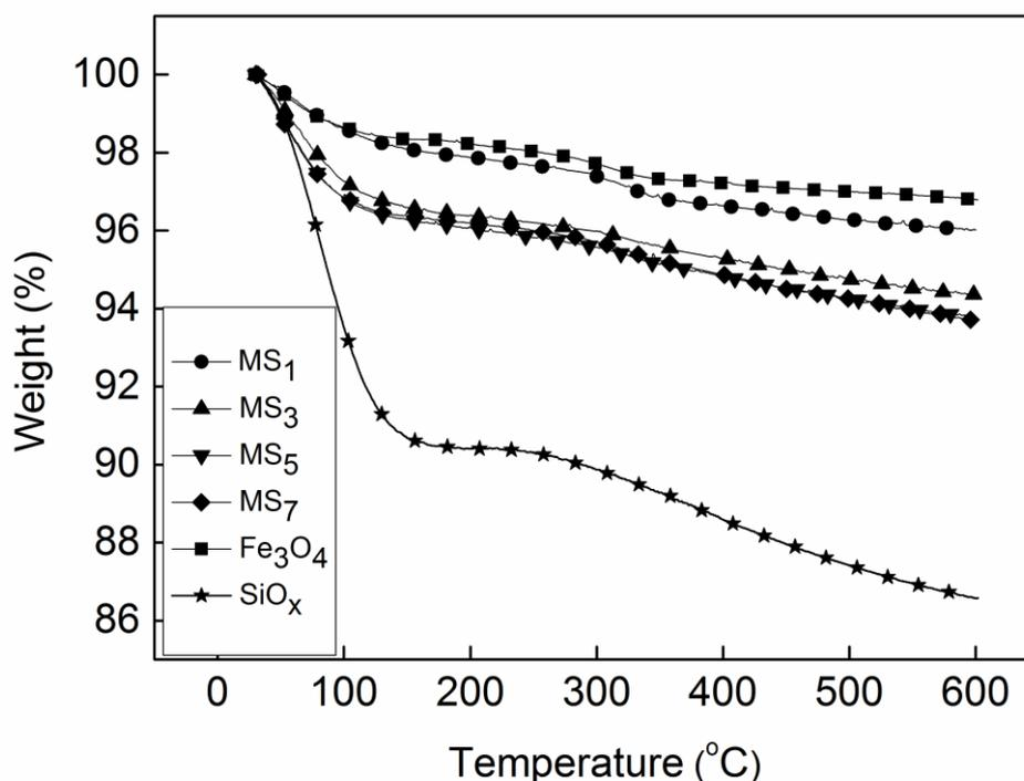
Fig. 3-2. TGA results for  $\text{Fe}_3\text{O}_4$ ,  $\text{SiO}_x$  and  $\text{Fe}_3\text{O}_4/\text{SiO}_x$  prepared with different amounts of TEOS. Samples were heated from room temperature to 600 °C with a scanning rate of 10 °C/min in flowing nitrogen gas
