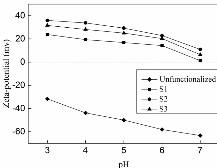
Fig. 4-2. Variation of zeta potential of three functionalized magnetic nanospheres and unfunctionalized magnetic nanospheres with pH
