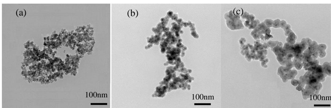
Fig. 3-4. TEM images of (a)  $\text{Fe}_3\text{O}_4$ , (b) FMS and (c) FMS-GA-EN. (Magnification 50 k)
