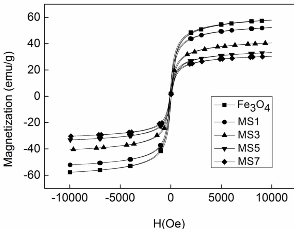
Fig. 3-3. Magnetic behaviors of Fe<sub>3</sub>O<sub>4</sub> and Fe<sub>3</sub>O<sub>4</sub>/SiO<sub>x</sub> prepared with different amounts of TEOS
