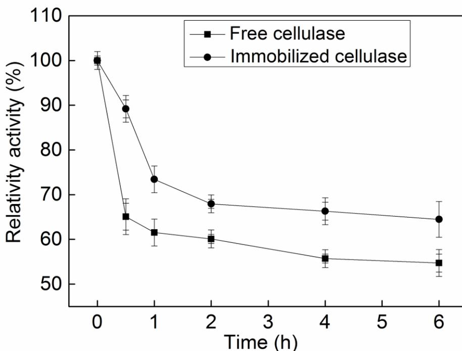
Fig. 3-8. Thermal stabilities of free and immobilized cellulase. CMC substrate was hydrolyzed by free cellulase and immobilized cellulase at 70 °C for 6 h
