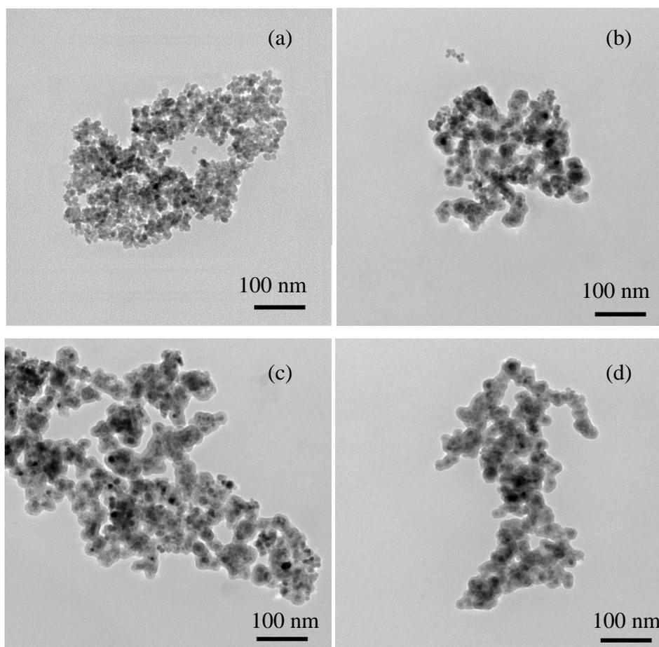
Fig. 4-1. TEM images of (a) Fe<sub>3</sub>O<sub>4</sub> and three functionalized magnetic nanospheres: (b) S1, (c) S2 and (d) S3
