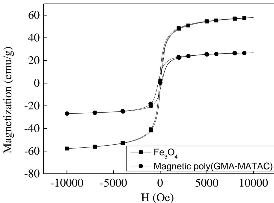
Fig. 5-4. Magnetic behaviors of (a) Fe<sub>3</sub>O<sub>4</sub>, (b) Magnetic poly (GMA-MATAC)
