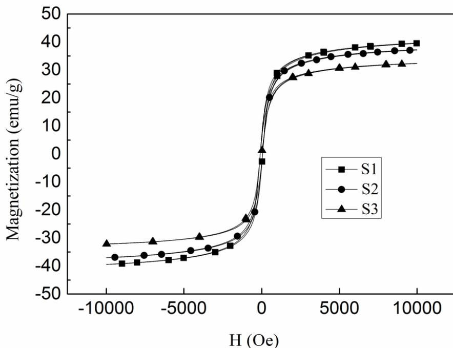
Fig. 4-4. Magnetite behavior of three functionalized magnetic nanospheres.
