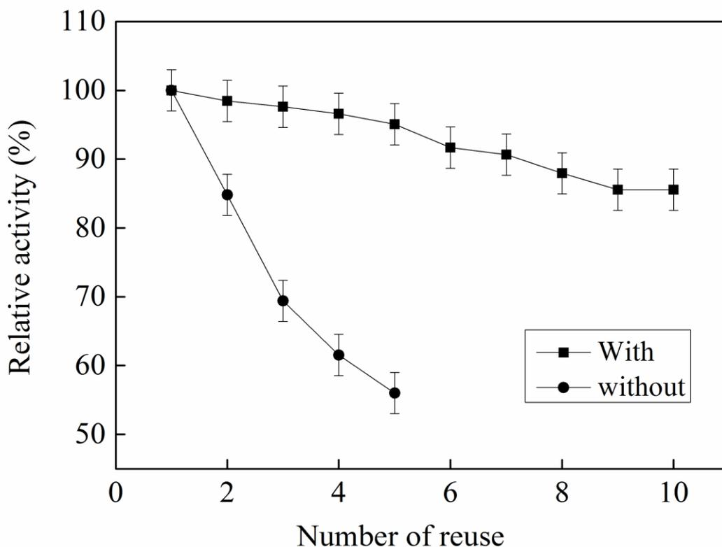
Fig. 4-11. Effect of immobilization method on reuse of immobilized cellulase. CMC substrate was hydrolysis by immobilized cellulase at 50 °C
