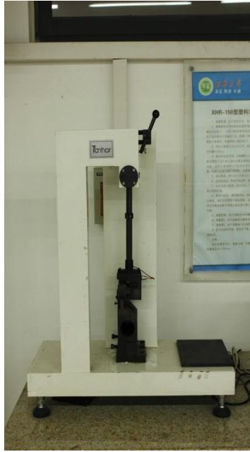
Fig. 2-13 Pendulum impact tester.
