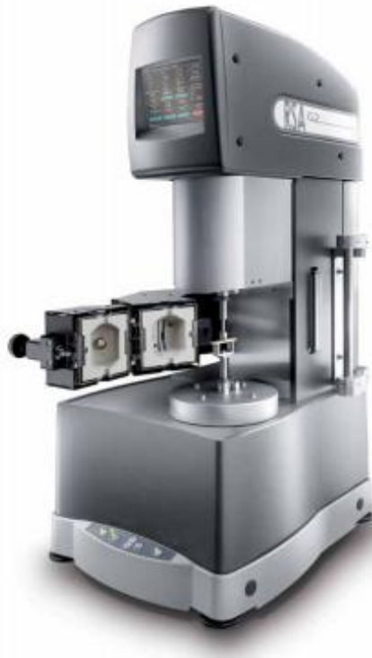
Fig. 2-10 Dynamic mechanical analyzer [16].
