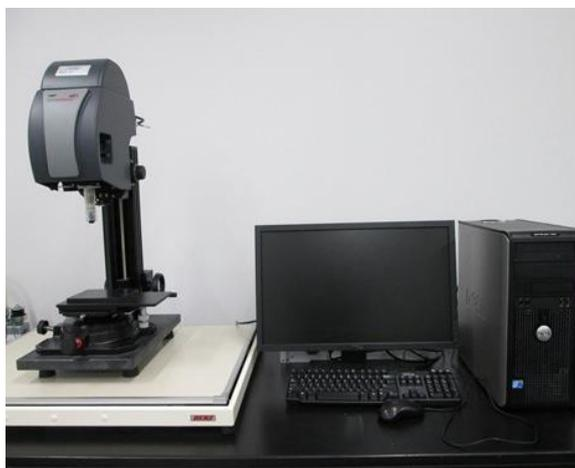
Fig. 2.3 Zygo New View 600 interferometer
