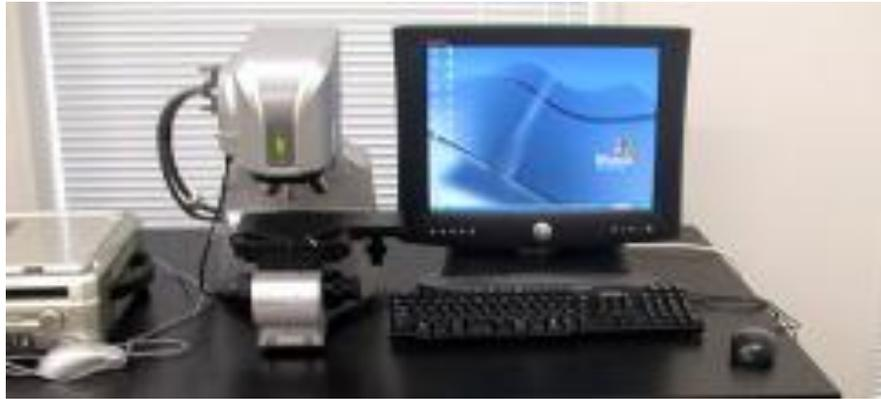
Fig. 2.5 Color 3D Laser Scanning Microscope, VK-8700
