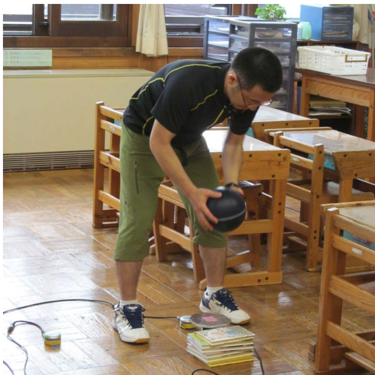
Photo 9. Picture of impact ball falling.
