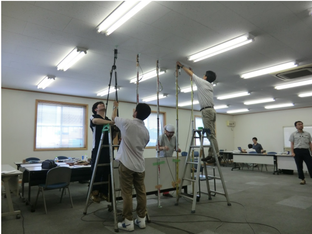
Photo 8. Picture of measuring the deflections of parallel chord trusses.
