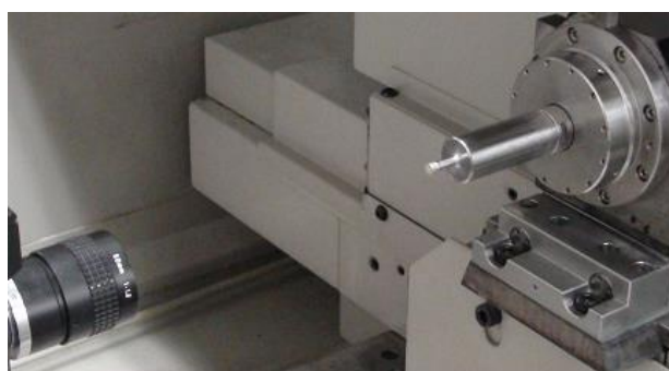
Fig. 2.7 UV amplitude measurement method.
