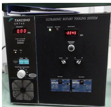
Fig. 2.3 Ultrasonic spindle controller
