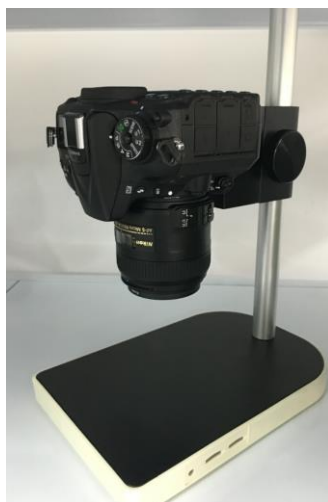
Fig. 2.3 Micro-focus digital camera
